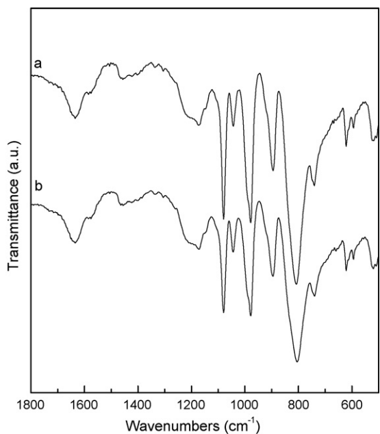
Fig. 8. The FT-IR spectra of (a) fresh 1 catalyst, (b) recovered 1 catalyst after the seventh run.
